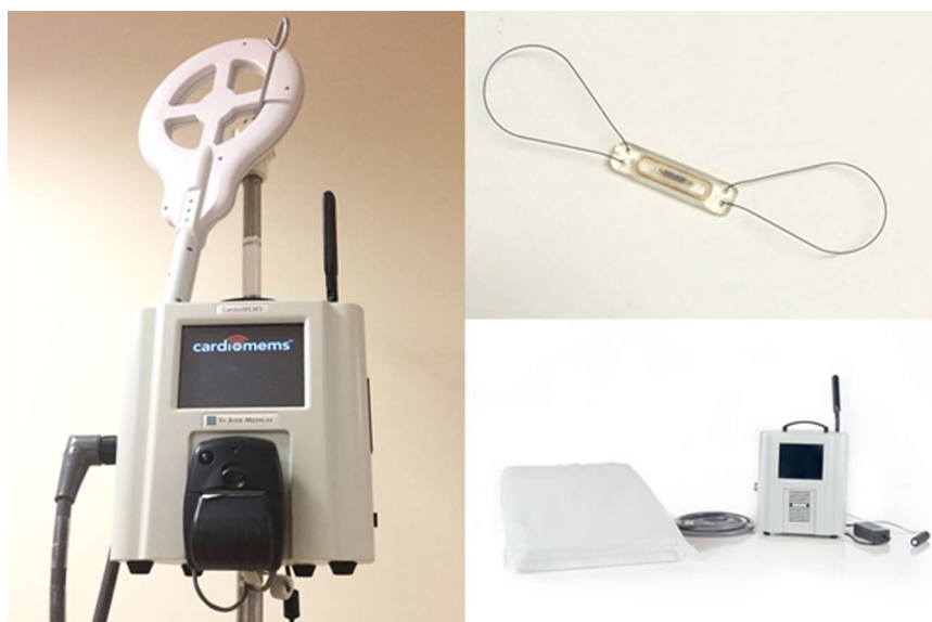
Figure 1 The CardioMEMS Heart Failure System Comprised of Implanted Wireless Sensor, Hospital Remote Unit and Home Remote Unit with Cushion.
