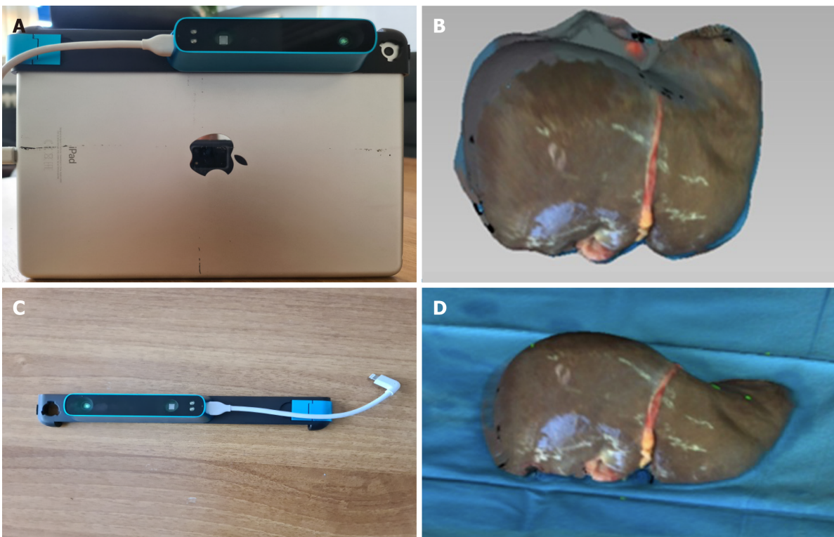
Figure 2 The particular sensor can be adapted to any device with iOS and iPadOS operating system. A: The device used in the present study. The structure core sensor, the adjustment bracket, the USB communication cable, and the iPad (6 th generation) are shown; B: The Occipital original structure sensor; C: An exported 3D model of a liver graft; D: The final 3D model of the liver graft.
