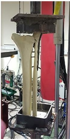
**Figure 3 Fibula pro-tibia construct of ankle fracture sawbone model mounted on the electromagnetic test frame (MTS 858 Mini-Bionix test machine, MTS Corp, Eden Prairie, MN, United States).**
