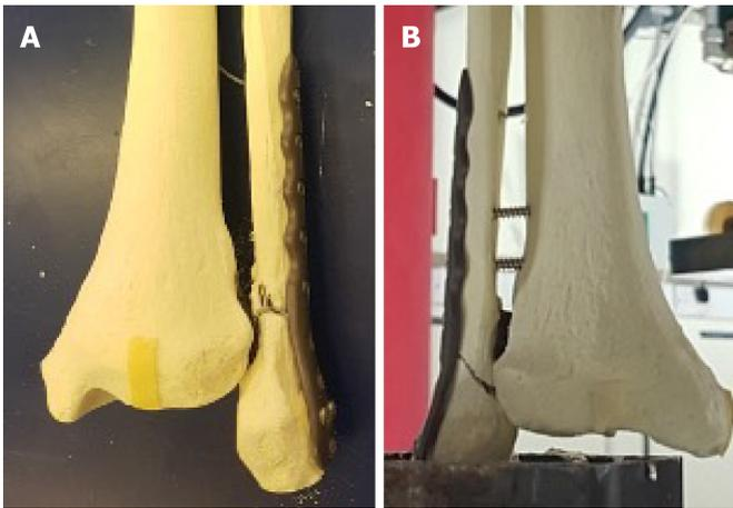
**Figure 2 Sawbone lateral malleolar fixation construct.** A: Sawbone lateral malleolar fracture treated with standard locking plate; B: Sawbone lateral malleolar fracture treated with locking plate in fibula pro-tibia configuration.
