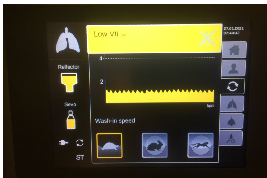
Figure 5 Display of the MIRUS™ controller. Yellow alarm refers to a low tidal volume. In this case, the wash-in speed “tortoise” should be selected.
