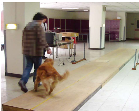
Figure 1 Gait analysis platform. The platform was a 10 m × 1.22 m × 0.19 m wooden walkway and in the middle of which embedded a pressure sensor. During the analysis the dog was leash-walked by its owner from one end toward the other end of the walkway. The walking speed was recorded by two sets of photoelectric cells. The walk was repeated until three valid speeds were recorded for each leg.
