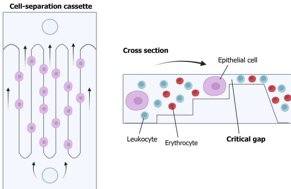
**Figure 6 Parsortix® PC1 system.** This platform is a physical method for detecting circulating tumor cells from a blood sample, suitable for subsequent user-validated downstream analyses. It incorporates single-use cell separation cassettes, allowing blood to pass through until reaching a critical gap where circulating tumor cells are captured. Citation: The authors have obtained permission to use the figure from BioRender.com (Supplementary material)[210].
