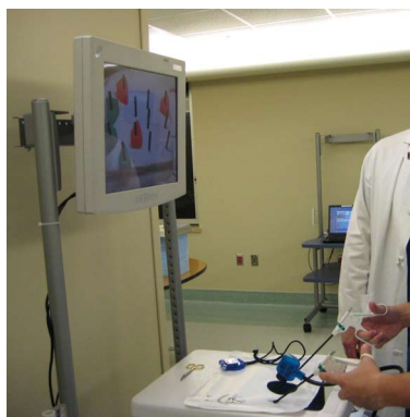
Figure 1 A camera and LED lighting system provide visualization and the surgeon works through two trocars placed in fixed positions through an opaque cover on top of the box.
