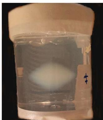
Figure 1 The photo of PAGAT polymer gel dosimeter.
