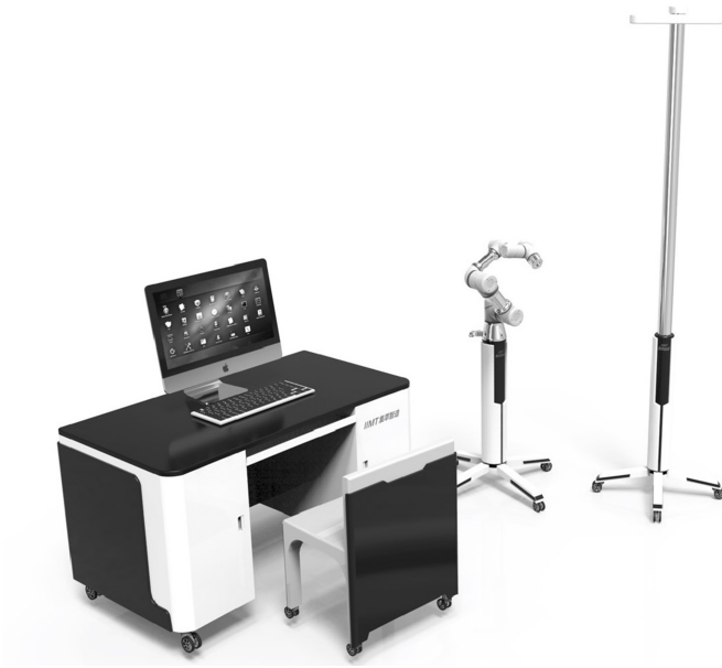
Figure 1 Schematic diagram of the binocular-stereo-vision-based navigation robot. The navigation robot was composed of binocular stereo visual tracking equipment, an operation planning and controlling system and a six-axis robotic arm.
