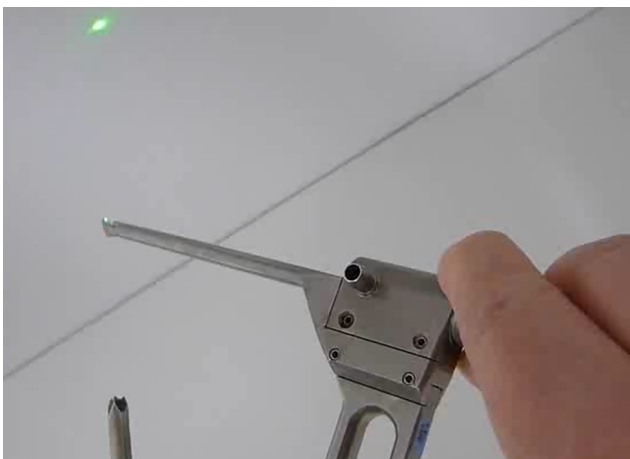
Figure 4 Reflected beam identifying the proper position on the extension of the pin.
