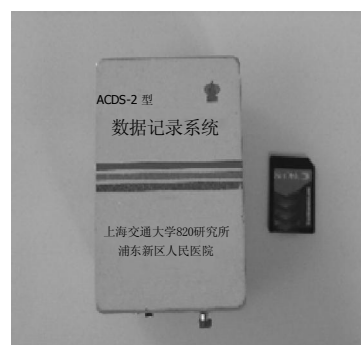
Figure 4 Data recorder and flash memory card. Left, data recorder; right, flash memory card.
