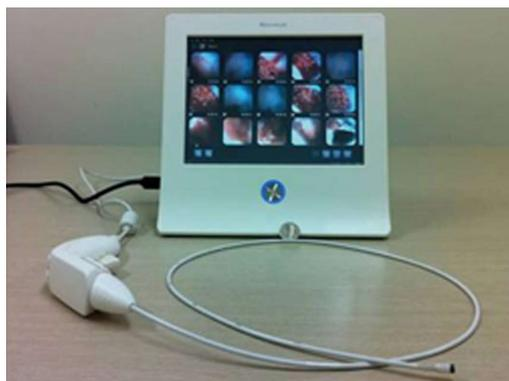
**Figure 1** EG scan device. The EG scan (version I) is composed of a disposable optical probe, a handle, and a display monitor.
