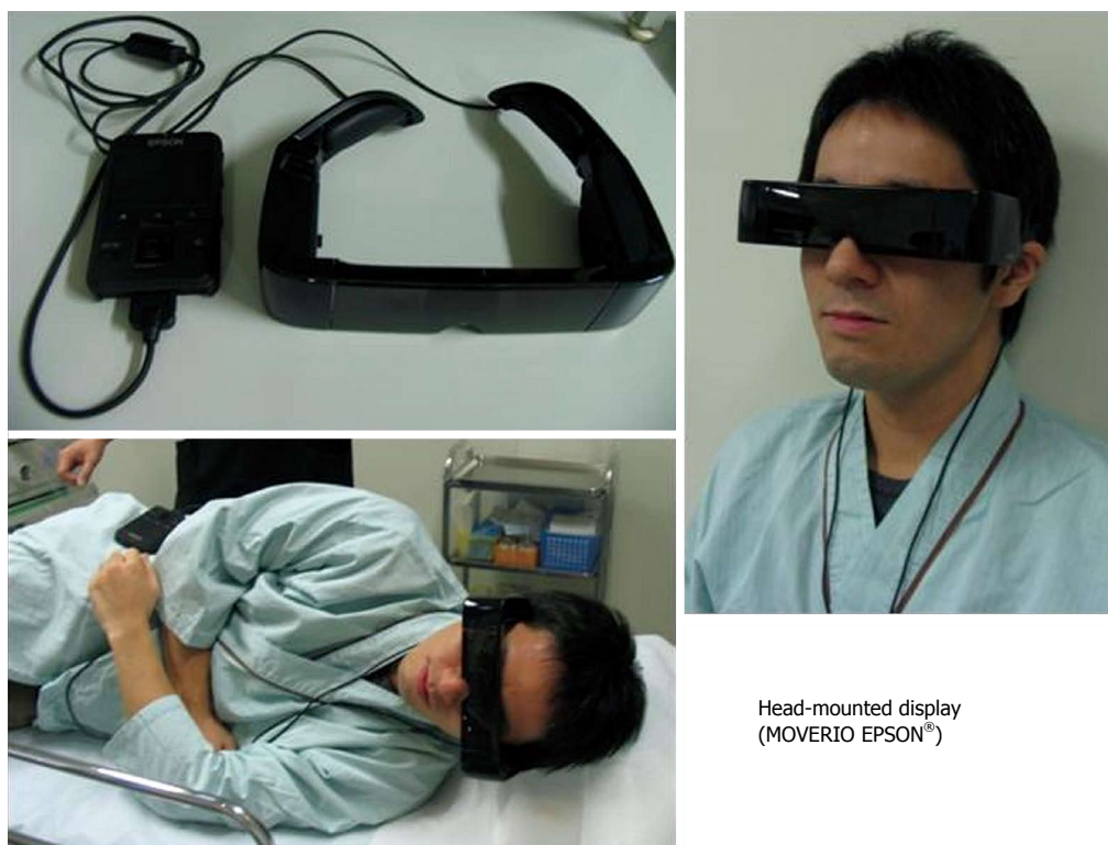
Figure 1 Head-mounted display (MOVERIO EPSON®; SEIKO EPSON CORPORATION, Nagano Japan) projects an image visible only from the inside without blocking the patient's vision.
