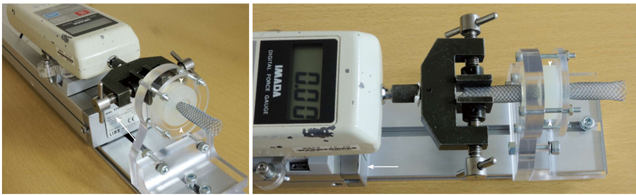
Figure 1 Resistance force to migration measurement machine. The machine consists of a retraction robot (arrows), a silicone wall (arrowheads), and a force gauge (Model DPRSST, Imada, Tokyo, Japan). The covered self-expandable metal stent is fixed into a round hole in the silicone wall (arrowheads) and its distal end is connected to the force gauge device. The stent is retracted from the wall at a speed of 1 mm/s. by using the retraction robot (arrows).
