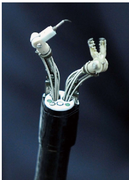
Figure 8 The MASTER system is a robotic arm system that can be mounted onto a conventional endoscope. Phee et al [68] , 2012.
