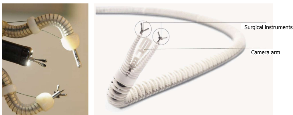
Figure 10 The Endomima system can be mounted onto a conventional endoscope. The arms allow passage of conventional flexible instruments. Each arm has up to 3 DOF of movement (Endotools Therapeutics). Roppenecker et al [129] .
