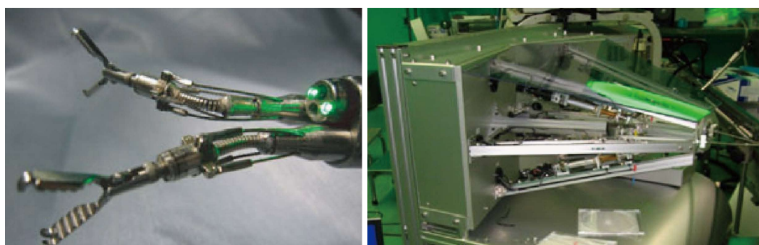
Figure 11 Scorpion like endoscopic robot is an externally mountable robot arms system. It is actuated by external actuators through traction cables (right). Suzuki et al [74] , 2010.
