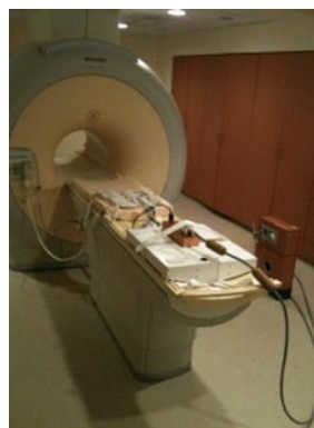
Figure 3 Equipment integration for magnetic resonance imaging-guided ultrasound therapy. Frontal oblique view of the 3T Philips MRI scanner with an 8-channel cardiac MR coil on the anterior part of the scanner table and ultrasound transducer on the posterior part of scanner table. MRI: Magnetic resonance imaging.
